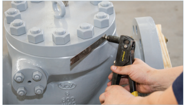
Riveting identification tag on Full Port Swing Check Valve
