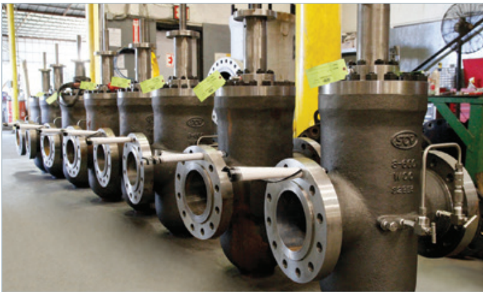
8" 600 Thru Conduit Expanding Gate Valves completed hydro testing
