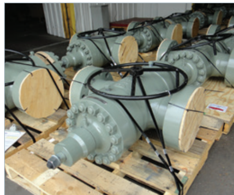
Palletted 7-1/16" 5000 PSI Thru Conduit Gate Valves ready for shipping
