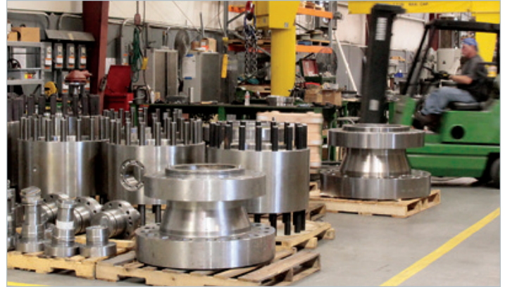
Stainless steel Trunnion Ball Valve components at Texas Operations facility
