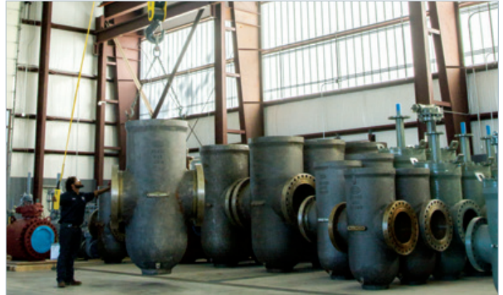
Thru Conduit Gate casting inventory stage for assembly
