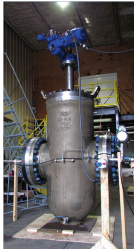
Shell TAT test on 24" 600 Thru Conduit Expanding Gate Valve
