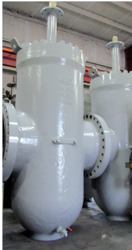
30" 600 Thru Conduit Expanding Gate Valves
