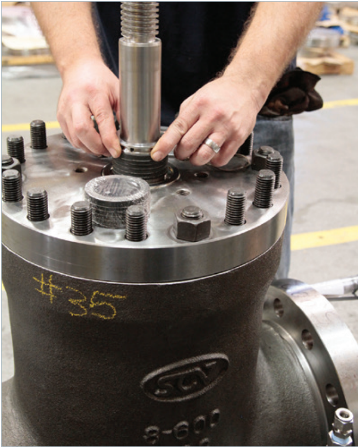
Installing packing into Thru Conduit Gate Valve
