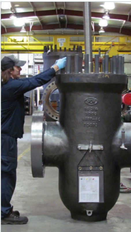
Assembly of an API 6A 16-3/4", 5,000 PSI Thru Conduit Gate Valve
