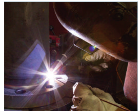
Welding flange to yoke tube
