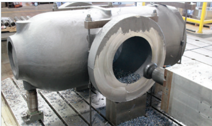
Machining 18" 600 Thru Conduit Gate Valve body
