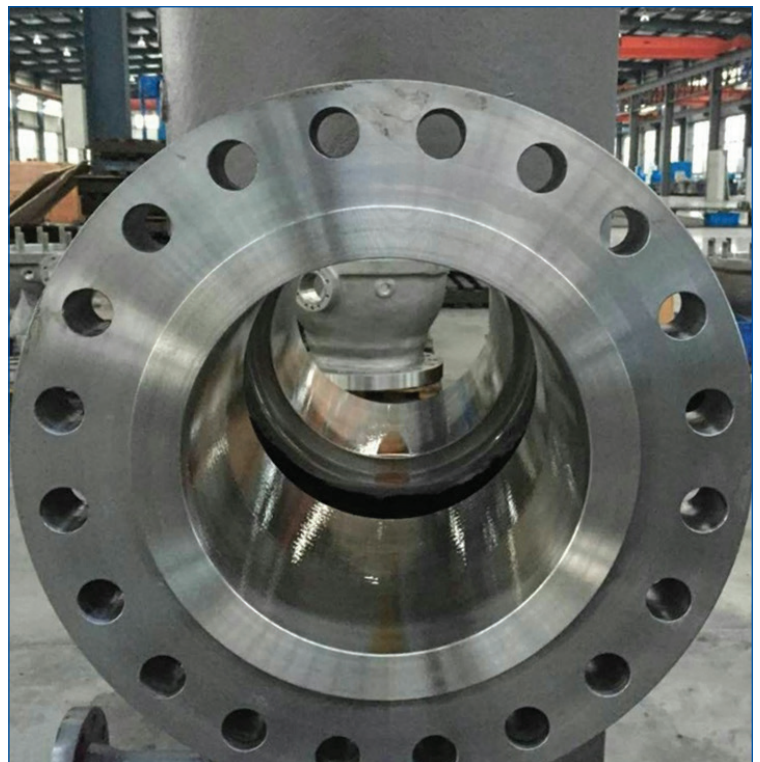
Bore & Flange Sealing Face - Inconel 625 Overlay
