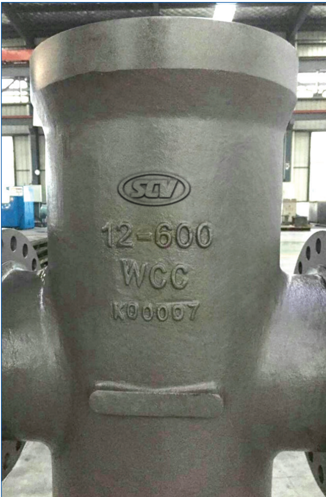
12" 600 Class Geothermal Body
