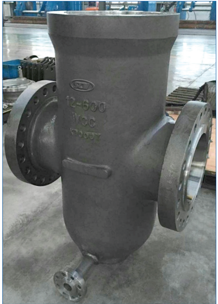
2" Flanged Body Drain Connection
