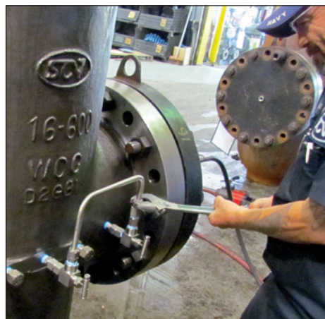
SCV Valve installed Thermal Relief system on 16" Class 600 Thru Conduit Expanding Gate Valve.
