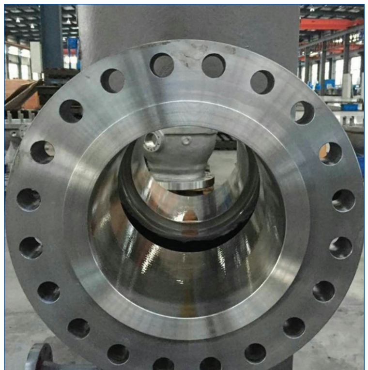
Bore & Flange Sealing Face - Inconel 625 Overlay
