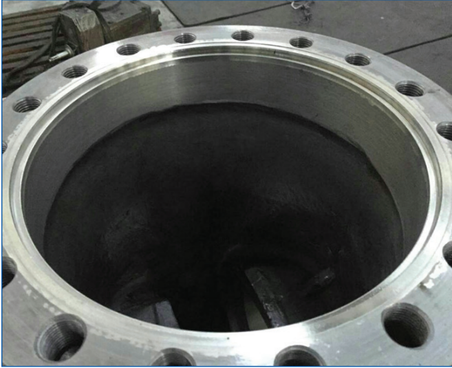
Body/Bonnet Connection - Inconel 625 Overlay
